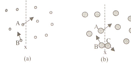
Figure 9.3 The difference between the Boltzmann kinetic formulation (a) and the Enskog formulation (b). In the Boltzmann formulation, heat flows across the interface at x only when the molecules (such as A) go across the interface. Molecules such as B do not contribute momentum and heat flux across x . In the Enskog model, even though B does not go across x , it collides with C and momentum and energy are transferred across the interface. This transfer occurs at a distance D and can be considered as due to the potential interaction between B and C.
